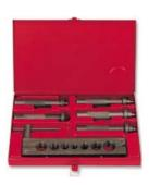
The holes in the die have a 90° chamfer on one side for forming tapered flanges with the turn pin.
